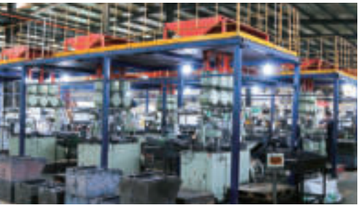
自动上料平台 Automatic Feeding Platform 设备作用： 帮助高速装配机上料，机械组装链条 The automatic feeding platform helps the high-speed assembly machine to load and mechanically assemble the chain
