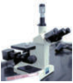
日本金相显微镜 Japanese Metallographic Microscope 设备作用： 检测分析链条及其系统件的金相组织 Detect and analyze the metallographic structure of chain and system parts
